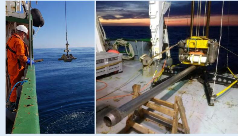
Fig. 2 (Left): (Action shot) Shipek grab sampler in use off the South-West coast of Cork. (Right): Vibrocorer stored safely ready for use during the AggreWind research cruise (CV18034). Barrel length 3 m; diameter 11 cm.
